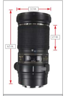
SPECIFICATIONS: 180mm (178.18mm tested), f/3.5 (f/3.46 tested), 14 elements in 11 groups. Focusing turns 150 degrees clockwise. Diagonal View Angle: 14 degrees.
